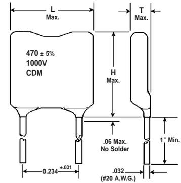
Ideal for snubber and RF applications, CDV16 mica capacitors now handle  $dV/dt$ s up to 275,000 V/ $\mu$ s and they assure controlled, resonance-free performance through 1 GHz.
