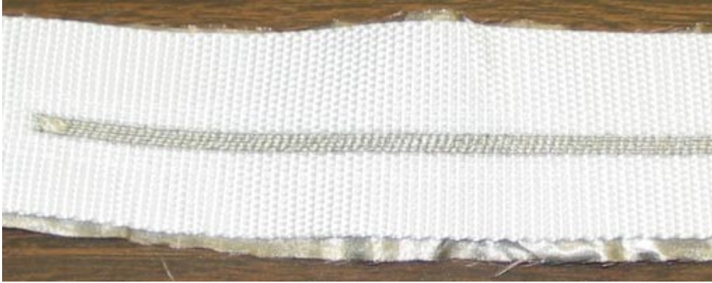
Figure 2. Fabric microstrip circuit with conductive fabric on nylon belt.
